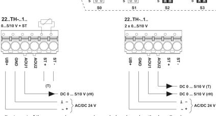
the adjustment of the measuring ranges is made by changing the bonding jumpers the output value in the new measuring range is available after 2 seconds
